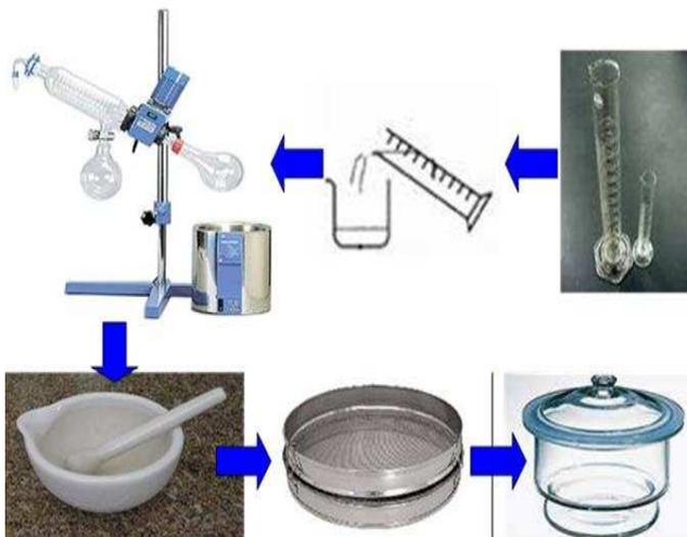
Figure 2. Attainment technique of solid dispersions by evaporation method in rotatory evaporator
