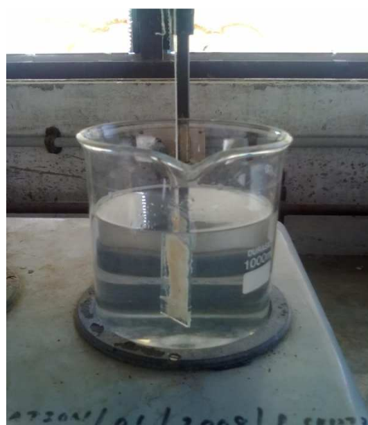
Figure 1. Schematic presentation of In Vitro Wash Off Test to Assess Mucoadhesive Properties
